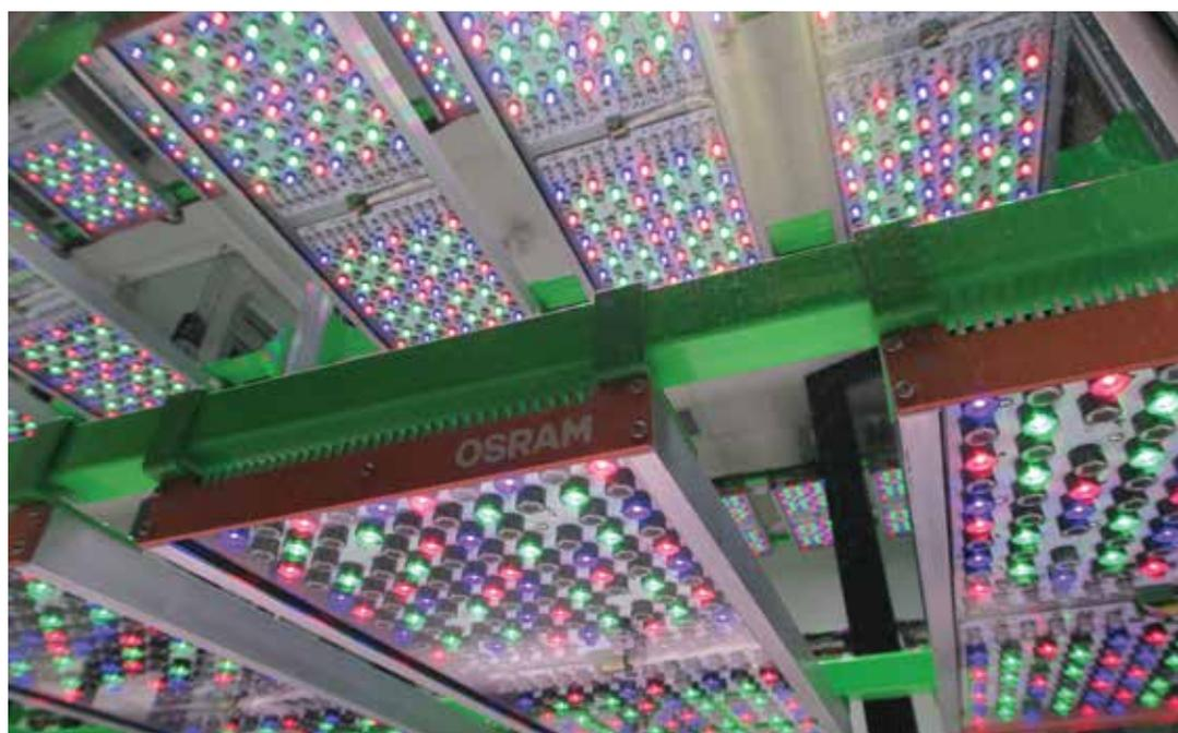
**Figure 1.** The quality of sole-source lighting, which refers to the spectral distribution of radiation, controls plant growth. Shown are LED fixtures in the Controlled-Environment Lighting Laboratory (CELL) at Michigan State University. For more, visit [www.hrt.msu.edu/labs/cell](http://www.hrt.msu.edu/labs/cell). (Photo: Qingwu Meng)
