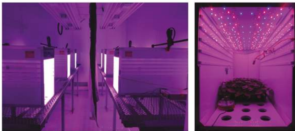
Figure 1. Experimental setup for indoor lighting treatments included six customized LED growth modules located in a refrigerated walk-in growth chamber (left). Seedlings were grown inside each LED growth module under the lighting treatments described in Table 1 (right).
