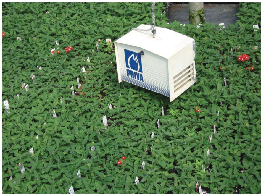
Figure 1. Air temperature should be measured in an aspirated box positioned very close to the plant canopy and away from wall, aisles and heating pipes.
