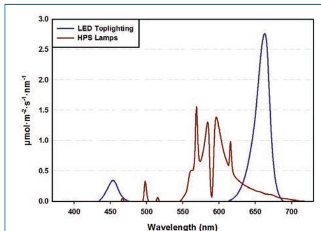
Figure 1. Spectral quality delivered from either light-emitting diode (LED) toplighting or high-pressure sodium (HPS) lamps at a photosynthetic photon flux (from 400 to 700 nm) of 70  $\mu\text{mol}\cdot\text{m}^{-2}\cdot\text{s}^{-1}$  at canopy level.
