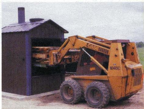
**Fueling an outdoor furnace can be as simple as loading a pallet of wood waste into the firebox twice each day. Photo courtesy of Heatmor, Inc.**
